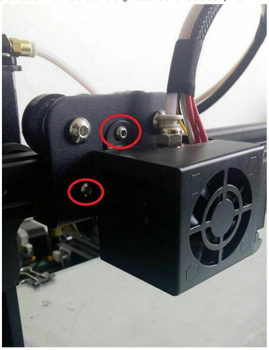
(2)Align the auto-leveling sheet metal parts with the nozzle assembly holes to ensure that the assembly ring of the auto-leveling sheet metal part is parallel to the platform, and then tighten the screws.
