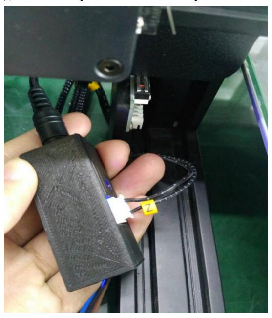
(5)The proximity switch can be adjusted by turning the screw to adjust the sensing distance of the proximity switch sensor. When the proximity switch senses an object, the sensor light will emit red light.
