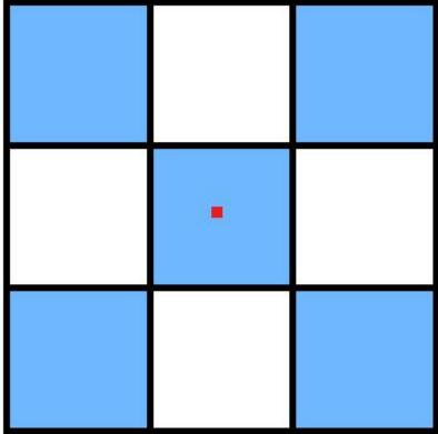
(2)After the auto-leveling Auto home, the function of the Level bed option will show on the operation interface. This is the basic auto-leveling function. The design based on the software code starts to measure the actual distance between the nozzle and the platform at each measuring position on the platform.
