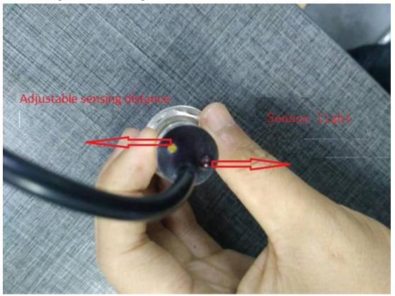
(6) Connect the power adapter to 100~240V power supply, and connect the automatic leveling plate box so that the nozzle just stop on the hot bed, and then install the auto-leveling sensor with voltage type, which must be higher than the nozzle in order to avoid that the model will be scraped while printing and make the state above the auto-leveling sensor indicates that the red light is just on. This is how the auto-leveling module is assembled.
