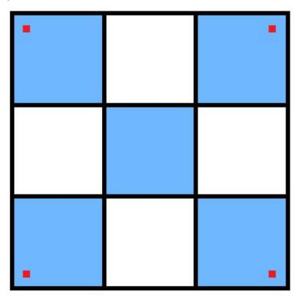
(3)Automatic leveling printing function, add the automatic leveling command G29 in the slicing software, Z-axis will automatically adjust to make the auto-leveling compensation printing according to the actual distance between the nozzle and the hot bed platform at each measuring position while printing for the better printing effect
